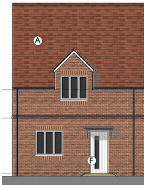
Figure 2: Terrace of four showing dentil course to eaves; projecting band course and cant brickwork under windows and headers above windows.
