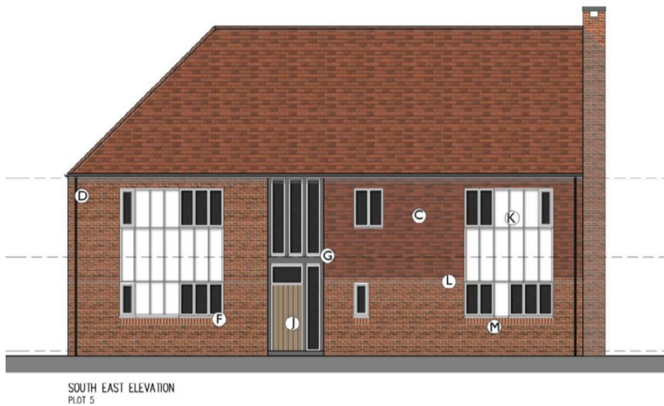
Figure 3: Barn like building form to show softer more local colouring: Blend of red/orange stock facing bricks and plain clay vertical hanging tiles. Powder coated white composite aluminium /timber windows.
